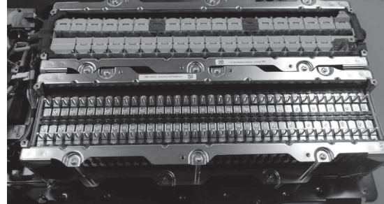
(b) Internal configuration of C-MAX hybrid battery pack
